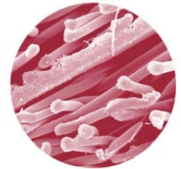
SlopeShield triple layer spun bond polypropylene
